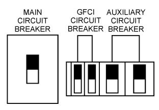
Figure 51. Main, AUX. and GFCI Circuit Breakers (ON)
